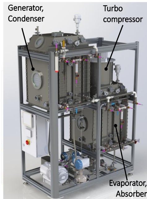
Figure 1: Design of the lab-scale hybrid chiller (Schweigler, 2019).
